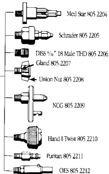
NOTE: Inlet on flowmeter is  $\frac{1}{8}$ " NPT F
